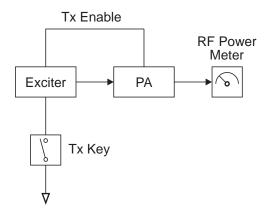
Figure 3.1 Test Equipment Set-up
